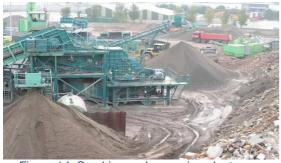
Figure 14. Crushing and screening plant
