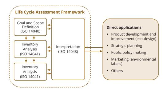
The LCAs undertaken here followed the **ISO 14040/14043** standards and utilised the **Ecoinvent** 3.6 database and the SimaPro 9.2 software. Three LCAs were carried out to compare five substitute materials (CDW, EAF, fly ash, GBF, M-Sand) and river sand in different applications in the construction sector:
